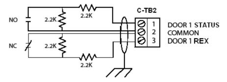
The figure above shows standard 2,200 ohm resistors. The NetAXS-123 panel accepts 1,000, 2,200, 4,700, or 10,000 ohm values. Note that both resistors must have the same value.
